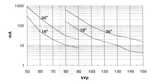
Figure 1-2. mAs vs. kVp, Minimum Requirements (Typical Single Phase X-ray Unit)
