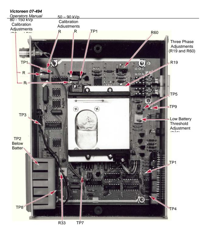
Figure 5-1. Adjustment and Test Point Locations
